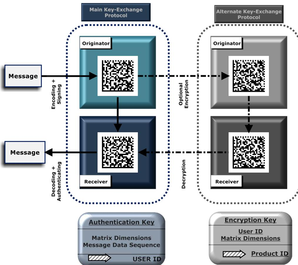
Both Authentication and Encryption keys are calculated using Random Number Generator (RNG) that uses all the data shown above as the input parameters. The length of this data string
